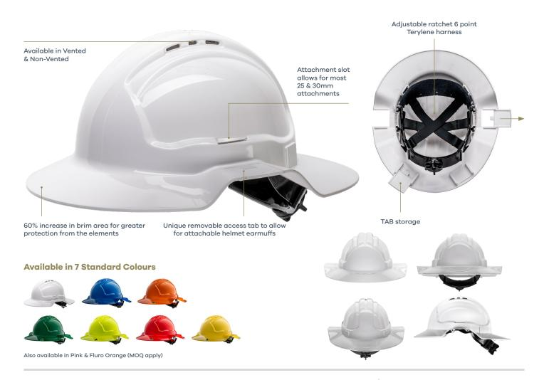
NEW, innovative designed broad brim hard hat. This new design includes greater protection from the elements including a 60% increase in brim area and 30% more protection, compared to current broad brim designs and 300% more brim area than a standard peak cap. The new Broad Brim hard hat has a unique removable access tab to allow for cap attachable helmet ear muffs. These tabs can be parked in the rear of the hard hat to prevent loss.
